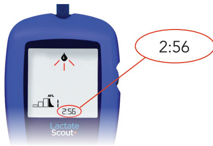
Display of the expired time following the last load measurement via the afterload timer
