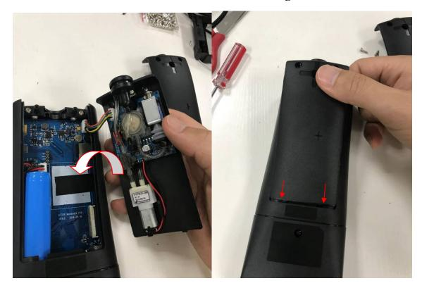
7. Install 2 screws and finish the exchange
