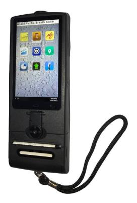
Model: AP-338 Version: The tester can remain accurate for 1 year of use. The more frequent the use, the more the unit will need to be calibrated. According to DIN31051, we recommend recalibration every 12 months (or earlier) basis to ensure maximum accuracy. OR exchange the factory pre-calibrated sensor module every 12months (or earlier)
