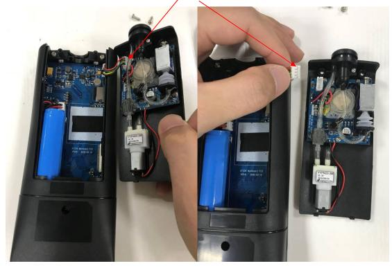
5. Plug the new Factory Pre-Calibrated Sensor Module to device
