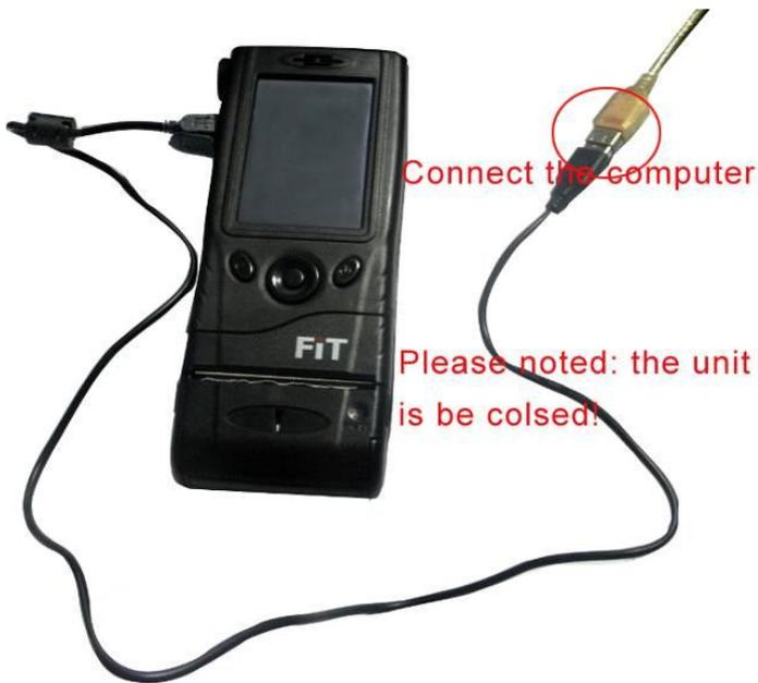
Step 1: Please turn off the FiT333 machine then use the download cable to connect the computer.
