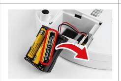
3. Remove the discharged batteries
