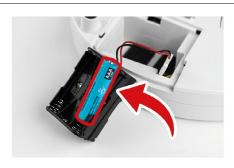
4. Insert the new alkaline batteries
