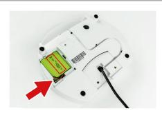
5. Insert the battery pack with the technical text facing upwards and the connector cable on the left. Insert the battery pack first and then gently place the cable in the bottom notch.
