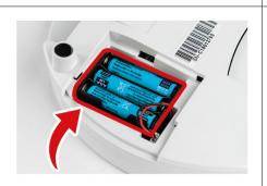
5. Insert the batteries container first and then gently place the cable in the bottom notch.
