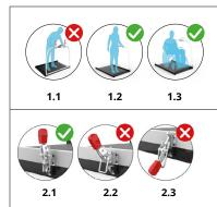
The function of the handrail is to assist the patient during ascent/descent, but it must not be used to hold on with one's full weight (1.1).
