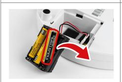
3. Remove the discharged batteries
