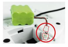
4. Connect the battery pack as shown in the figure
