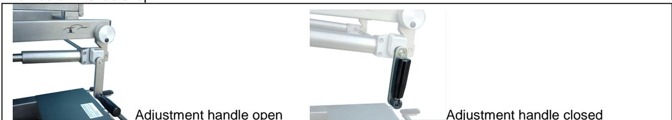
The trolley has as endowment a **revolution indicator** well visible placed in correspondence with the adjustment handle, instrument useful to immediately know the point of inclination reached and also to reach the position **0000** on the trolley indication, useful to proceed to the activity of taking over/deposit of the table top.
