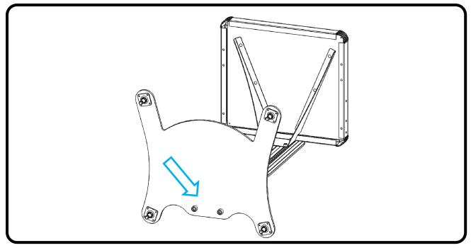
4. Put and fix the basis near the column with 2 screws TCEI
