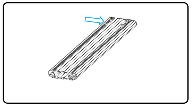
1. Put the column on the desk and unscrew 4 screws TCEI M6x10.
