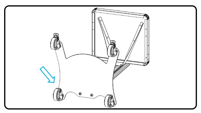
5. Insert the wheels into the pin under the basis.
