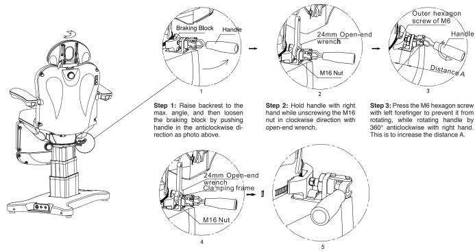
Step 4: Keep clamping frame horizontally by holding handle with right hand, while screwing the M16 nut with open-end wrench in the anticlockwise direction.
