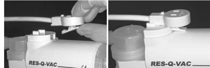
1. Insert the clip of the LED light source into the back opening of the adapter assembly and push forward until the narrow portion of the light slides into the top channel of the adapter assembly. Make sure the front lip of the light is resting under the two brackets on the top of the adapter assembly.
