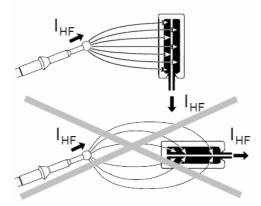
**NB** Current should flow in parallel to the body surface and never pass through the thorax. The patient must be placed on a dry and perfectly isolated surface. The patient must be kept isolated from conductive parts and the operating bed must be earthed. Use dry gauzes to avoid that different areas of the body come into contact with each other.
