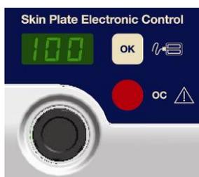
If the impedance value is accepted, the impedance indication is recognized and the display and OC indicator are extinguished. If the shown impedance is accepted, but the impedance increases respect the accepted value, the unit avoid the distribution, shows the OC condition, without acoustic signal (only present during distribution) and shows the new impedance value.
