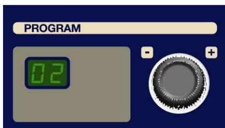
Using the section PROGRAM it is possible to store 16 different operational conditions and levels of output power.
