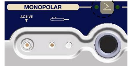
**Note:** For use foot-switch, press keys and view monopolar foot-switch light.
