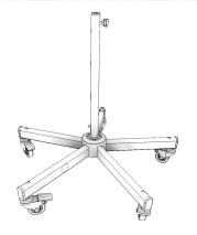
**WARNING:** Ensure the stem is tightly secured and that the base is stable and parallel to the floor. Verify that all wheels rotate freely.
