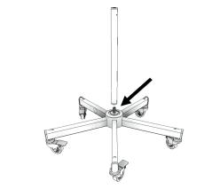
After assembling the base, position the upper base stem in correspondence with the M12x90 screw.
