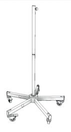
**WARNING:** Verify that the stem is tightly secured and that the mobile version is stable and parallel to the floor. Ensure that all wheels rotate freely.
