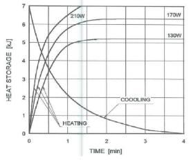
Anode Thermal characteristics
