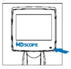
When the light switches from green to red, it indicates that the batteries are low. In this case, please change batteries.
