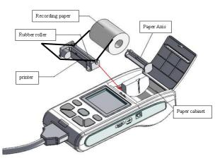
Figure 6-1 Installation of recording paper
