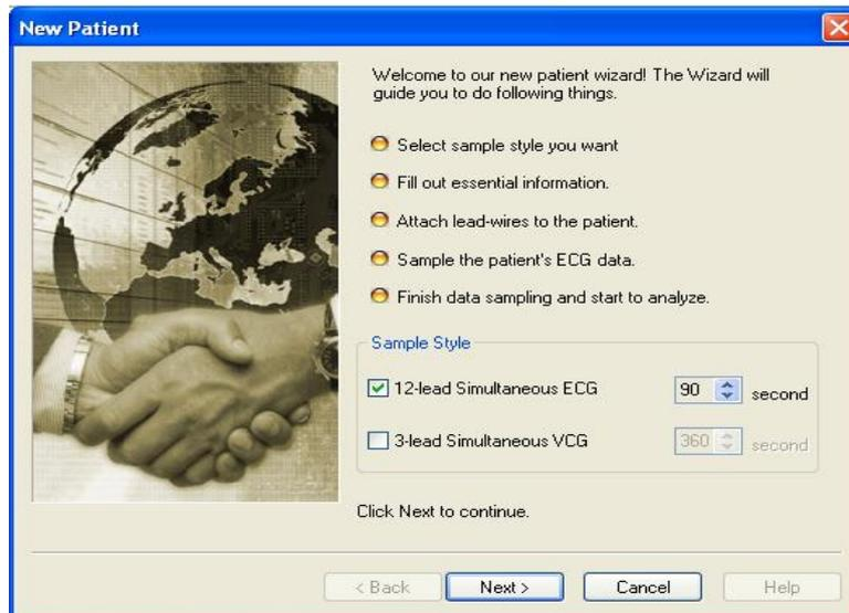
**12-lead simultaneous ECG:** You can change the sampling time according to your needs. But if you want to sample data for FCG (Frequency ECG), it is strongly recommended sampling 90 seconds.
