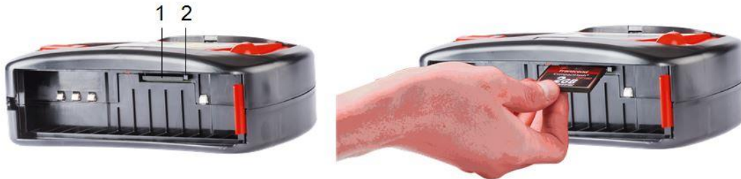
Fig. 8: Inserting / replacing the SaveCard
