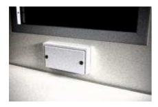
1) Remove the lid seals acting on the two screws by rotating with Allen key which is provided. Do the same action inside the booth.
