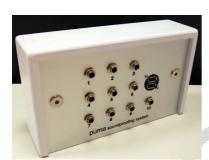
A tripolar jack connection plate is available on request. 10 jack inputs, suitable for most of diagnostic and clinical instruments.
