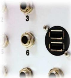
Additional double USB port to connect with other instruments or PC.
