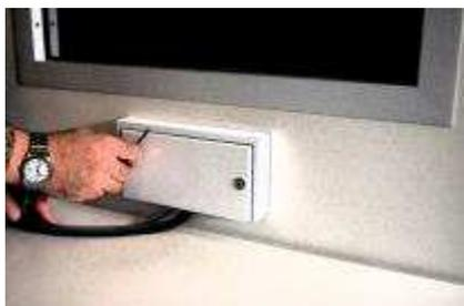
3) Once introduced them let them fall and close again by positioning the seal (external and internal) previously removed and tighten the Allen screws with the provided wrench.
