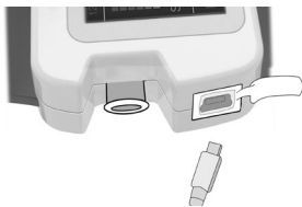
Figure 5.16 Sketch map for connection between Sleep apnea screen meter and USB data line
