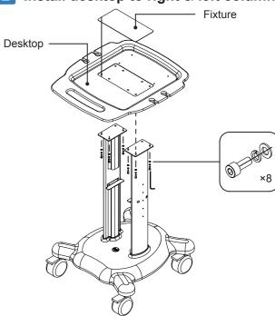
Put the fixture into the desktop, fix them with the left & right column together using 8 screws(M5×12) from bottom.
