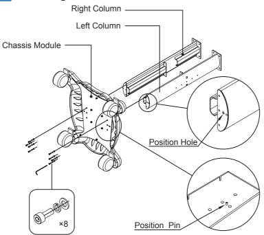
1.Insert the left column into the chassis module, position pin should be fixed in the position hole, assemble them together with 4 screws at the bottom of the chassis.
