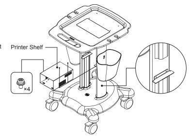
Fix the printer shelf into the corner support between 2 columns using 4 screws(M3×6).
