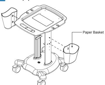
Hang the 2 paper baskets the screws side of the left & right columns. The height of paper basket locket can be adjusted by moving the
