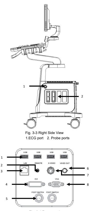
Fig. 3-4 Rear panel 1.USB 2.0 ports 2.Remote port 3.LAN port 4.DVI port 5.Foot Switch ports 6.Video Out port 7.S-Video port 8.VGA port
