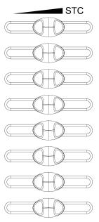
STC can be used for adjusting gain compensation in different image depth.
