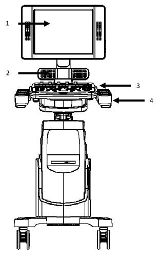
Fig. 3-2 Front Side View 1. Monitor 2. Speaker 3. Keyboard 4. Probe holder
