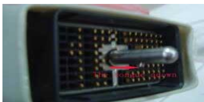
Fig. 3-5-1 Tongue of Probe connector
