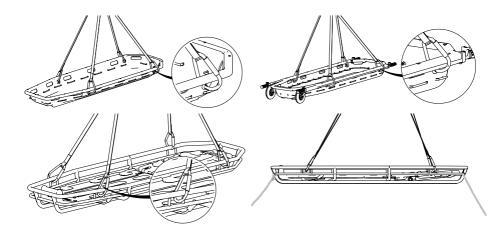
A Before lifting or lowering, after carrying out all the safety checks necessary for handling, adjust the harness and/or distribute the load inside the basket stretcher in order to balance its horizontal position when it is then handled.
