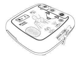
As the battery pack is inserted, the device starts a self-test. If the device status is normal, is shown on the Status LCD. If X is displayed on the Status LCD or flashes red or yellow on the Status indicator after the self test, please refer to [Chapter 8 : Troubleshooting] of these Instructions for Use.
