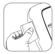
2. Insert a new battery pack in the direction of the arrow with the label facing upward as shown in the figure below.
