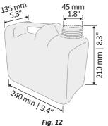
IMPORTANT NOTE! Pay attention to the size of the tanks to prevent breakage or damage to the suction lances.
