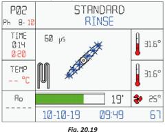
19) Disinfection phase begins: the machine will rise the water temperature to 90°C (194°F) and will keep it for 5 minutes.
