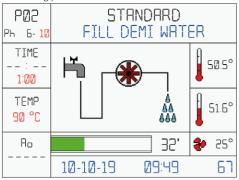
14) Rinse phase begins: the machine will rise the water temperature to the presetted value and will keep it for the presetted time.
