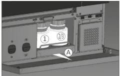
Fig. 11.1 TT model liquid containers
