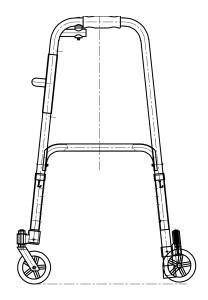
Install the front and rear casters assembly according to the direction of arrow in the image (note: casters assembly is divided into left and right).
