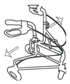
Open the folded "frame assembly" in the direction shown in the figure
