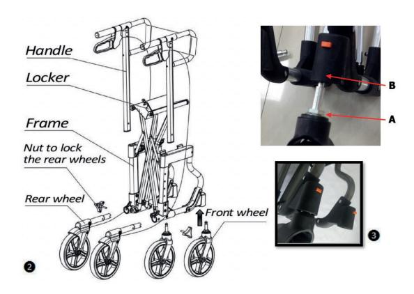
c) Fold the frame a little, then insert the handles into the frame (Figure 4), until the pins into the hole, then unfold the frame again.
