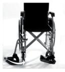
To install the footrests, align the holes in the supports with their pins on the wheelchair frame, and then rotate the footrest inward by correctly hooking the locking lever into the wheelchair frame. To remove, release the footrest lever from the wheelchair frame, then turn them outwards and pull upwards..
