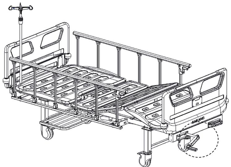
Use 2pcs 17-inch Allen wrenches to unscrew the telescopic rocker knot, take out the bolt, and replace the rocker. When the replacement is completed, install the bolts in the order shown in the figure, and use the wrench to tighten the knot.
