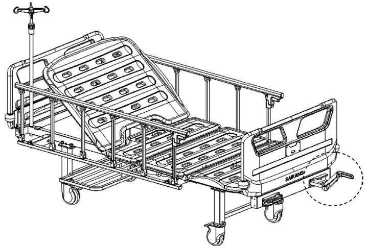
**Leg up and down: Pull out manual crank handle** and turn it counter clock wisely to lift the leg and turn it clock wisely to lower the leg.
