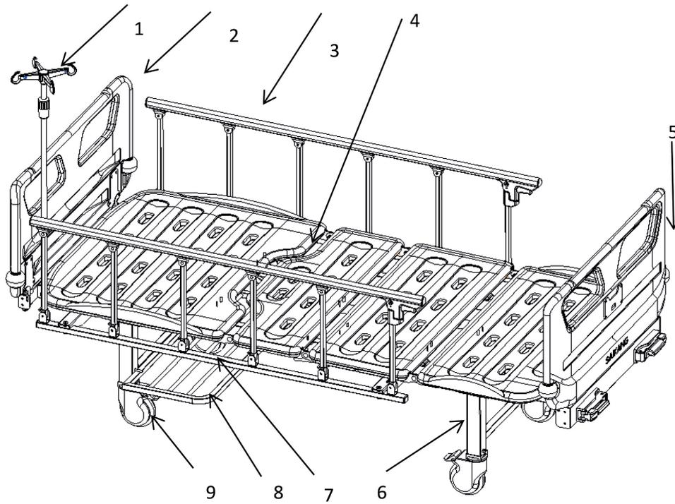
1-IV pole 2-Head board 3-Guardrail 4-Bed surface board 5-Foot board 6-Leg frame 7-Drainage hook 8-Shows holder 9-Caster
