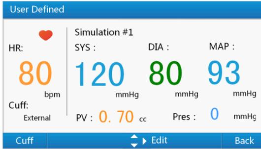
Figure 22 User defined BP simulation interface
