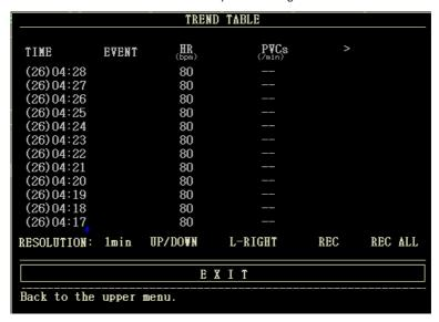
Time corresponding to each group of trend data is displayed at the leftmost list with date in brackets. Marked events are listed under the "EVENT" corresponding to the time of marking. Trend data of all parameter is divided into 8groups.
