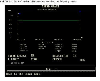
The y-axis stands for measured value and x-axis stands for time. The symbol " " in above figure is the cursor of trend graph. The value that the cursor points to, is displayed under the trend graph, and its corresponding time is displayed above the trend. Other trends except NIBP trend are displayed in continuous curves. In NIBP trend graph, the symbol "\*" represents the coordinate of the NIBP value.
