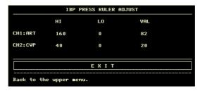
The waveform scale displays in the IBP waveform area, the three dotted lines from top to bottom respectively represent the upper scale, reference scale and lower scale of the waveform, which can be set, the steps are as followings:
