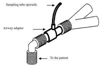
For intubated patients with an integrated airway respiration adapter in the breathing circuit: connect the luer male head on the sampling tube to the concave port of the airway adapter.
