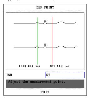
The ISO and ST are the two measurement points in ST segment, both of them can be adjusted. The reference point is the position where the peak of R-wave locates (as figure below). The ST measurement value for each heartbeat complex wave is the difference between the two measurement points.
