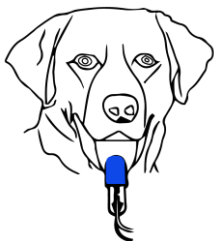
Figure 3.4 Clip the sensor on tongue
