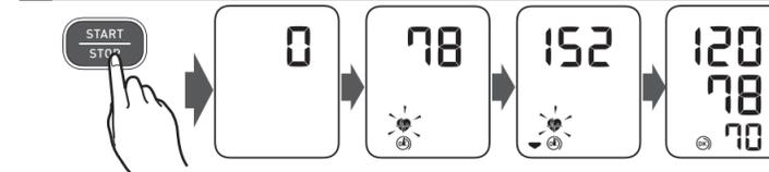
When the [START/STOP] button is pressed, the measurement is taken and saved automatically.
