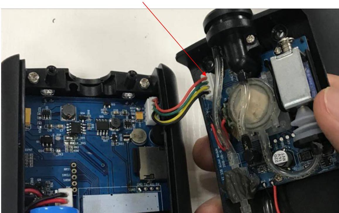
**6. Install the sensor module to Main device housing.**
