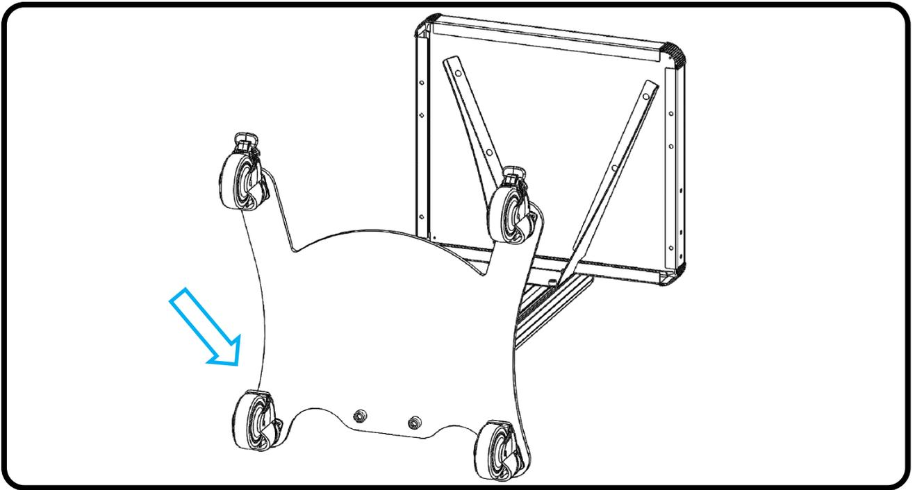
5. Insert the wheels into the pin under the basis.
