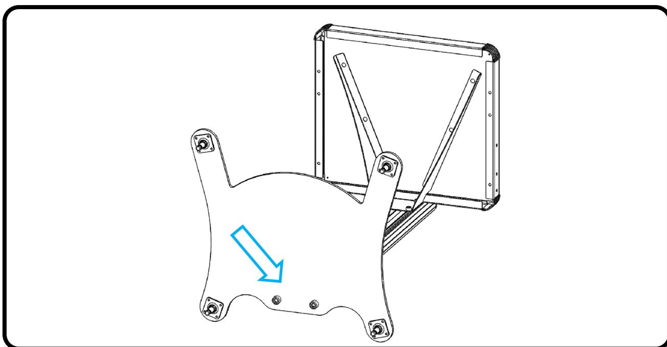
4. Put and fix the basis near the column with 2 screws TCEI M10x40.
