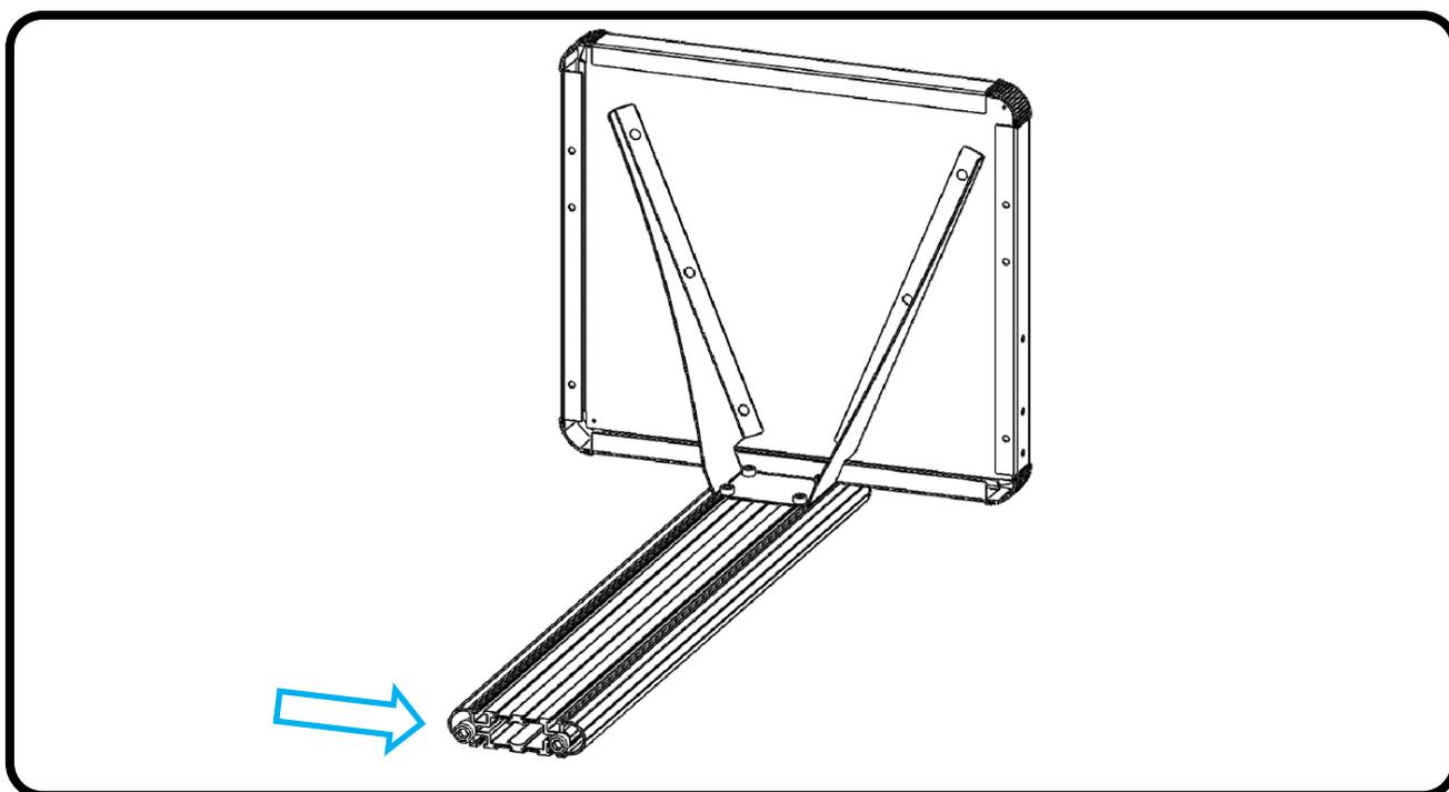
3. Unscrew 2 screws TCEI M10x40 under the column.
