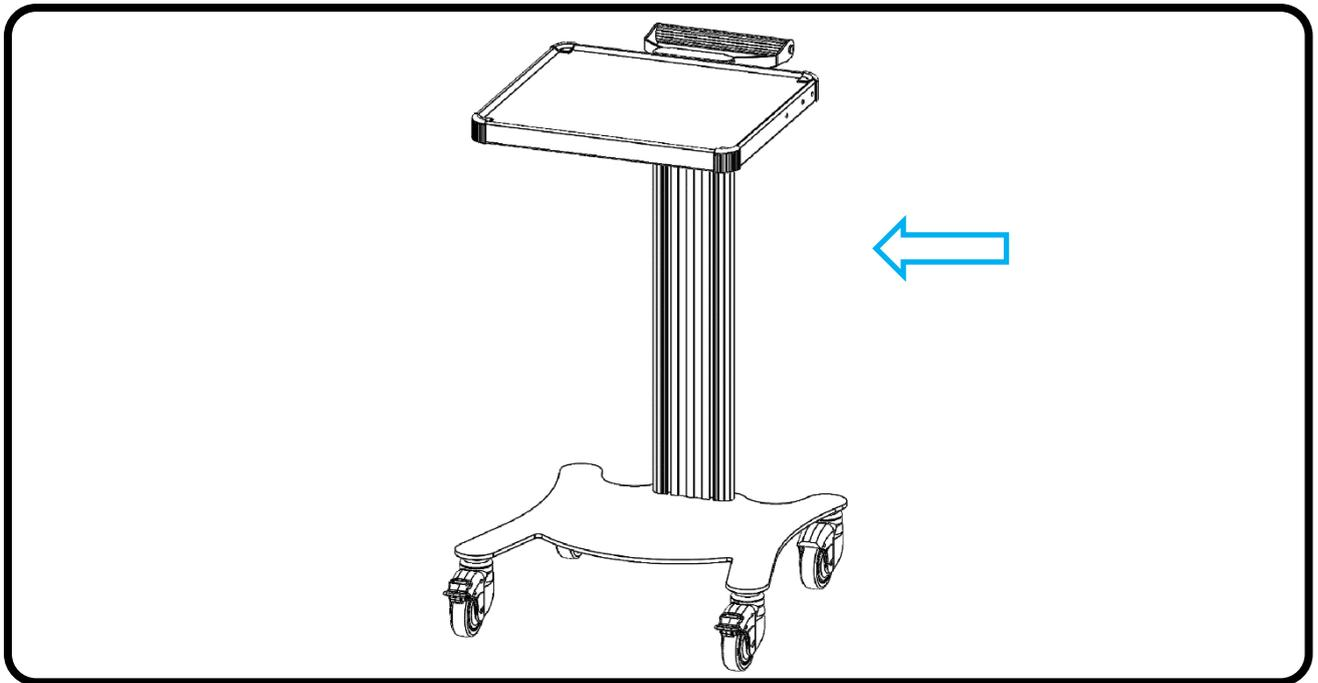
7. Put and fix the back handle from the rear of the column with 2 screws TCBEI M6x10. The trolley is ready for use. Good job.
