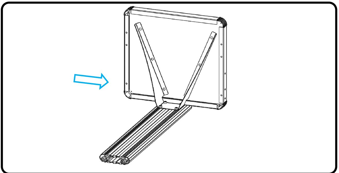
2. Put the shelves on the column and fix with 4 screws TCEI M6x10.
