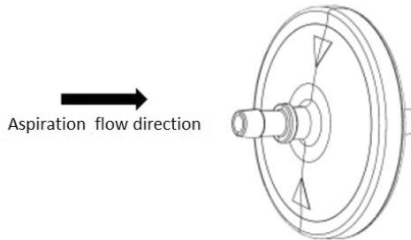
Make sure the filter is assembled with the arrows on the side of the patient.
