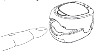
Figure 3 Put Finger into the Oximeter
