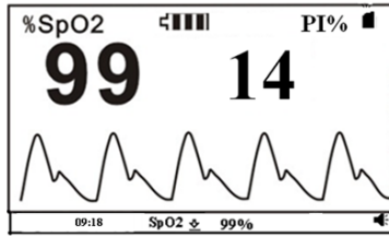
Figure 14 Display Screen with PI Value
