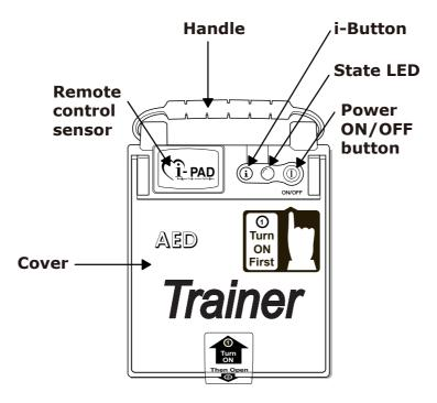
• Top View of the i-PAD NF1200-T with its cover closed
