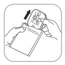
6. Plug the connector of the pads into the AED electrode pads connector port of the i-PAD NF1200-T
