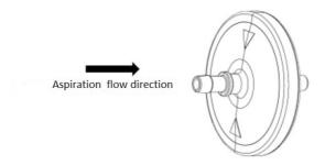
Make sure the filter is assembled with the arrows on the side of the patient.
