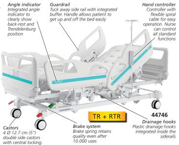
Anti-winding hard **TECHNICAL SPECIFICATIONS** 44746 44744 208.5x99.5 cm 208.5x102.5 cm Height adjustment: from 42 to 73 cm from 45.5 to 74.5 cm Mattress platform: 192.5x90 cm Safe working load: Back-rest adjustment: + 0-75° (± 5°) Knee-rest adjustment: 0-32° (± 5°) Trendelenburg: 0-12° 0-12° Reverse Trendelenburg Angle indicator: 0-90° 10+9 cm Auto-regression: Position line: 30° Motor: life: 20.000 movements under 50 dB 100-240 V - 50/60 Hz Voltage:
