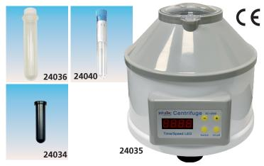
**RECOMMENDED FLUID SPEEDS AND TIMES** Fluid **Tube Size** Inserts Speeds Times None or Black Blood Large (6-15 ml) 5.000 rpm 5 minutes Small (3-5 ml) Blood White 5,000 rpm 6 minutes Microtubes (0.5-2.0 ml) Blood Green 5,000 rpm 7 minutes Urine 10-15 ml urine tubes None 2,000 rpm 5 minutes Fecals 10-15 ml fecal tubes None 1,700 rpm 6 minutes
