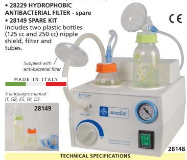
Regulator for suction intensity: max suction -0.33 bar (-248 mmHg) 220-230 V - 50/60 Hz - available on request 110 V - 60 Hz Operating voltage: Max flow (air litres/min): 14 l/min
