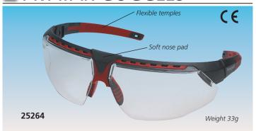
• 25264 AVATAR GOGGLES - black/red - fog resistant, antiscratch Anti-fog coating goggles provide anti-scratch performances to keep lenses clear and workers safe. Ultra-light and soft brow frame. 9 base lenses made of polycarbonate with hydroshield coating. Provided with innovative and adjustable nose pad. PPE Category II. Norms: EN 166, EN 170.
