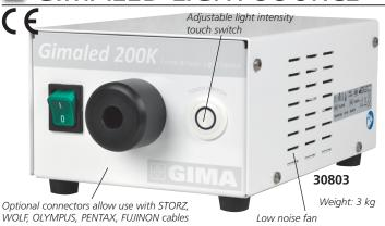
• 30803 GIMALED 200 K **LIGHT SOURCE - 16 LED** Compact, lightweight, powerful light source for endoscopic use. A low noise fan provides the necessary cooling inside the metallic structure of the light source. Touch switch enables a variable
