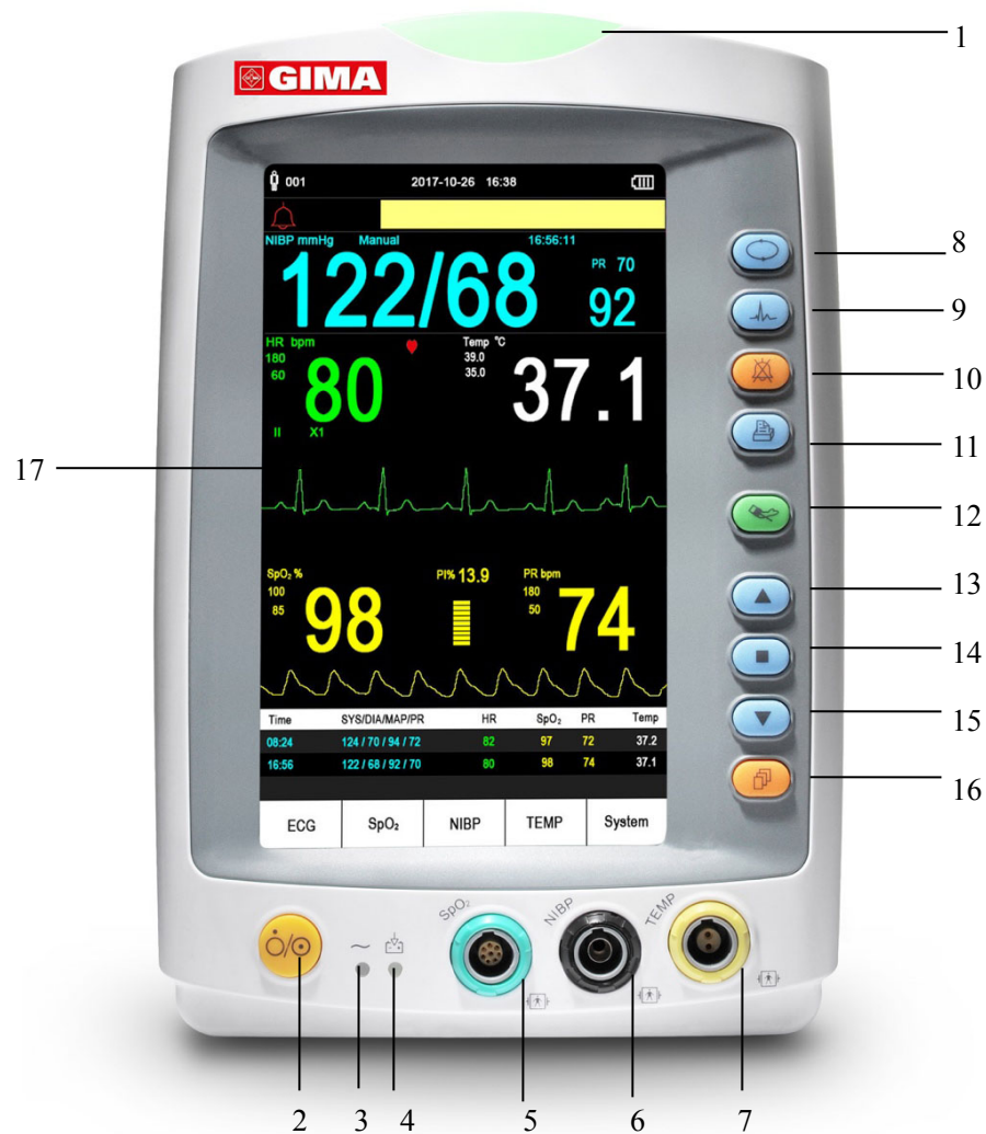
Figure 3.1B Front panel illustration for monitor (with ECG function)
