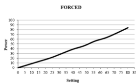
FORCED Output Power Diagram on Rated Load
