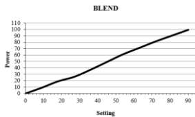
BLEND Output Power Diagram on Rated Load
