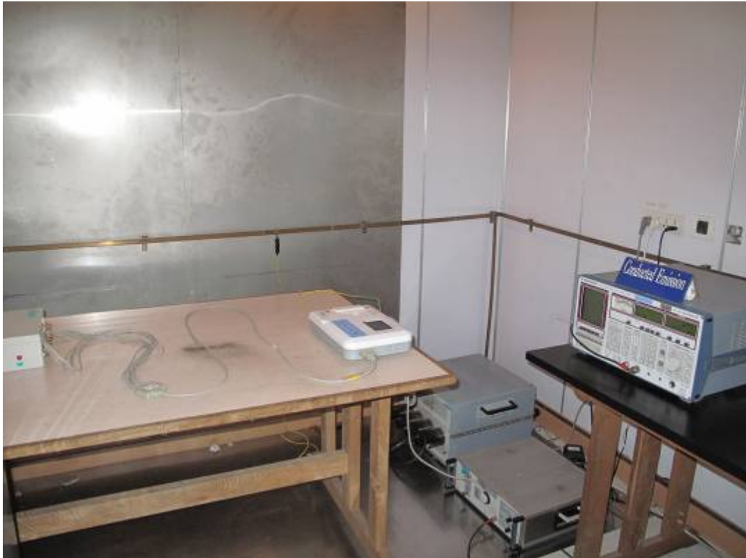
Photo of test setup for Mains Terminal Disturbance Voltage
