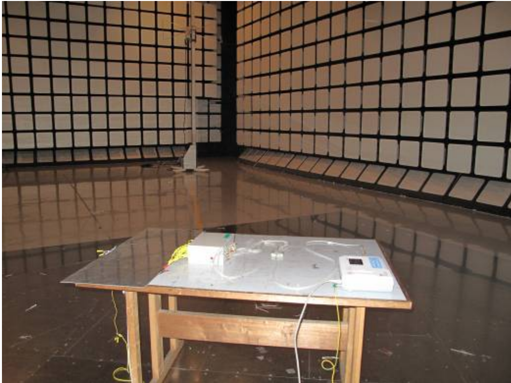
Photo of test setup for Radiated Disturbance
